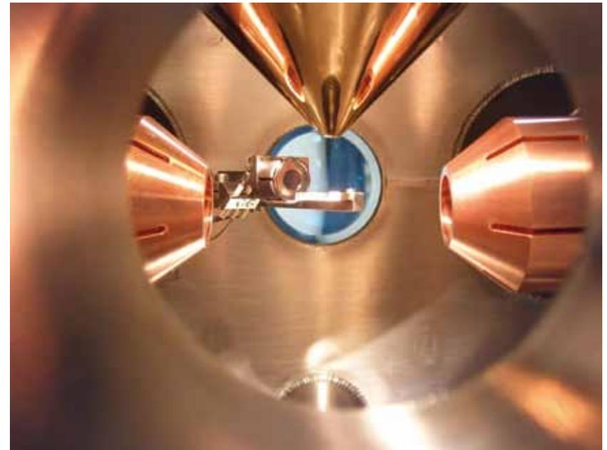
Inside view of the scanning electron microscope for ultracold atoms.
