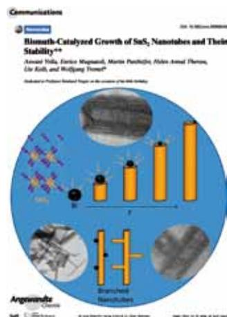
Scheme illustrating the VLS approach for the growth of SnS<sub>2</sub> nanotubes. Top row: (left) SnS<sub>2</sub> crystal structure. (right) Bi metal droplet catalyzing the growth of a SnS<sub>2</sub> nanotube. The growth of the nanotube grown depend upon the size of the liquid droplet. Nanotube growth stops when the Bi droplet is evaporated. Bottom row: Branched SnS<sub>2</sub> nanotubes grown from Bi droplets on the sidewalls of a parent tube.
