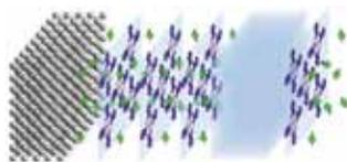
Schematic picture showing spin polarized electrons (green) injected from a cobalt substrate (gray) through different layers of the organic semiconductor copper phthalocyanine.
