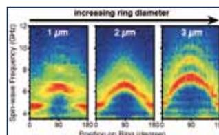
BLS spectra as a function of position on the ring structures. Red (blue) indicates high (low) spin-wave intensities.
