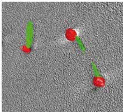
Projection of a reconstructed 3D TEM tomography representation of three CdS quantum rods (green) with a large gold domain (red). 3D tomography reveals the non-centric attachment of the gold domain on the semiconductor rod (best seen in this projection on the hybrid particle on the upper right).
