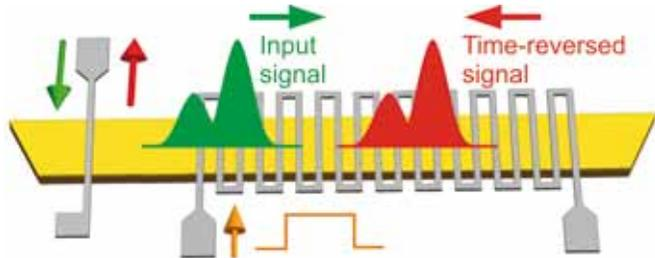
Turning back time. A signal wave (green) is launched from an antenna (left) and allowed to propagate into a structure known as a dynamic artificial crystal. By rapidly altering the properties of the crystal structure using a control pulse (orange), a time-reversed version of the signal (red) is created.
