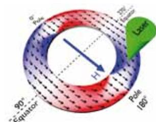
The black arrows indicate the direction of the magnetization in a micro-ring with a diameter of 2  $\mu\text{m}$ . The spin-wave intensity is locally probed by means of Brillouin light scattering (BLS) microscopy with a focused laser spot.
