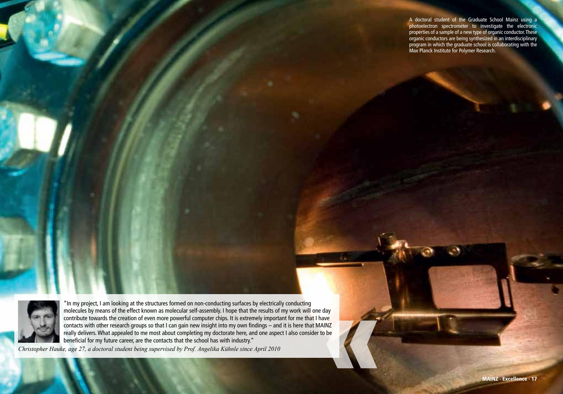
A doctoral student of the Graduate School Mainz using a photoelectron spectrometer to investigate the electronic properties of a sample of a new type of organic conductor. These organic conductors are being synthesized in an interdisciplinary program in which the graduate school is collaborating with the Max Planck Institute for Polymer Research.
