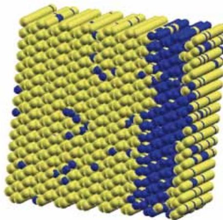
Distribution of In and Ga atoms in a Monte Carlo simulation. The snapshot shows phase separation into  $\text{CuInSe}_2$  and  $\text{CuGaSe}_2$  at low temperatures.
