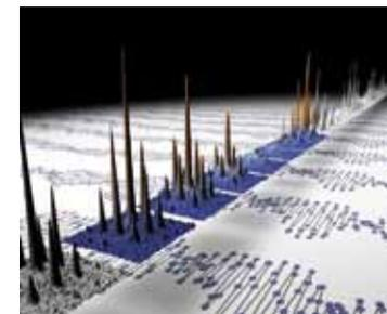
The collapse and revival dynamics of Bose-Einstein condensates trapped in an optical lattice reveal exotic multi-body interactions. The image shows a sequence of interference patterns containing the dynamics.
