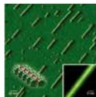
Non-contact atomic force microscopy image showing uni-directional wires self-assembled from heptahelicene-2-carboxylic acid molecules on the cleavage plane of calcite.
