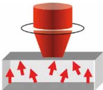
Schematic picture showing a laser beam illuminating a ferromagnetic sample. The randomly oriented red arrows (spins) in the sample represent the laser-induced reduction of ferromagnetic order.
