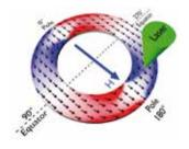
The black arrows indicate the direction of the magnetization in a micro-ring with a diameter of 2µm. The spin-wave intensity is locally probed by means of Brillouin light scattering (BLS) microscopy with a focused laser spot.
