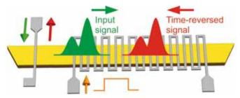
Turning back time. A signal wave (green) is launched from an antenna (left) and allowed to propagate into a structure known as a dynamic artificial crystal. By rapidly altering the properties of the crystal structure using a control pulse (orange), a time-reversed version of the signal (red) is created.
