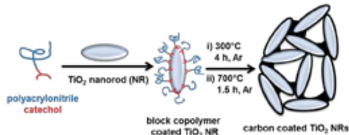
Fig.: Carbon coating approach of  $\text{TiO}_2$  nanorods using anchoring block copolymer carbon precursor.
