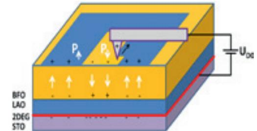
Fig.: Charge carriers are introduced locally into the electron gas at the interface by changing the ferroelectric polarization with a piezo force microscope.
