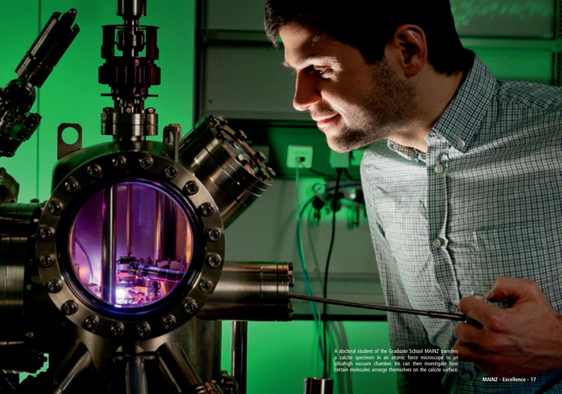
A doctoral student of the Graduate School MAINZ transfers a calcite specimen in an atomic force microscope to an ultrahigh vacuum chamber. He can then investigate how certain molecules arrange themselves on the calcite surface.
