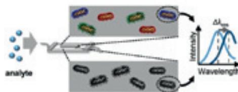
Fig.: Analyte detection with mapped (upper panel) and unmapped (lower panel) plasmonic nanoparticles
