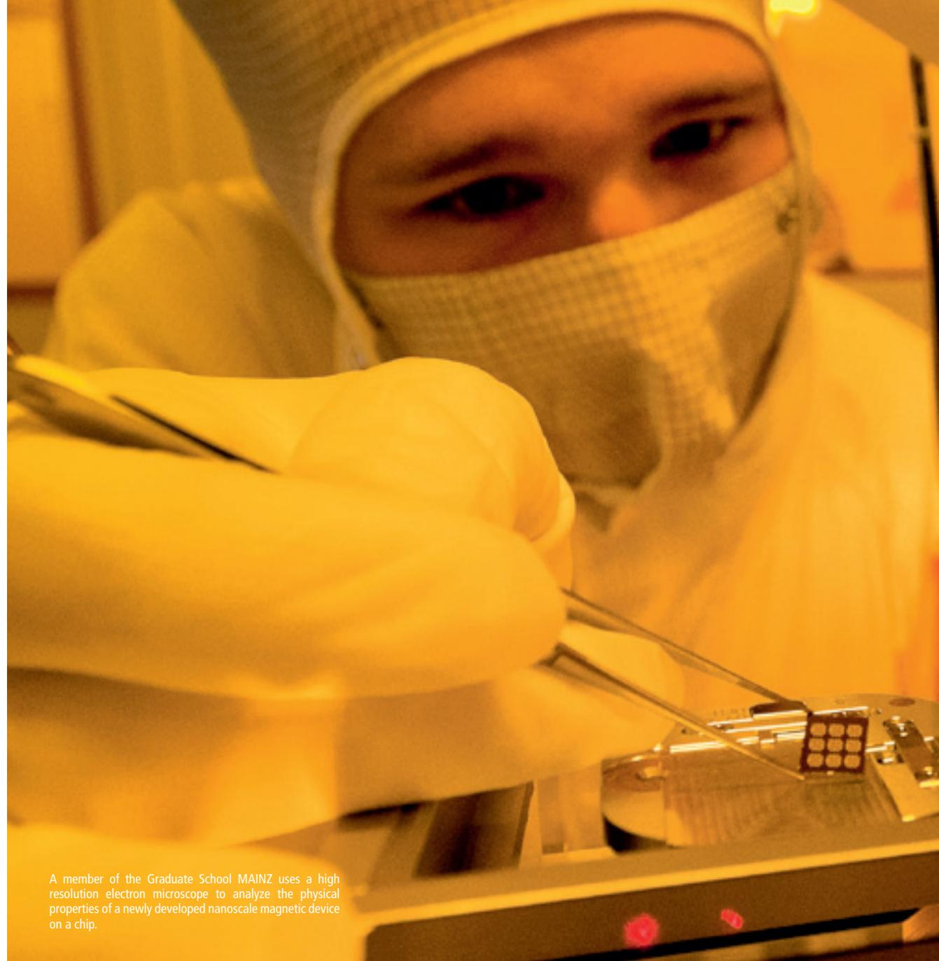
A member of the Graduate School MAINZ uses a high resolution electron microscope to analyze the physical properties of a newly developed nanoscale magnetic device on a chip.
