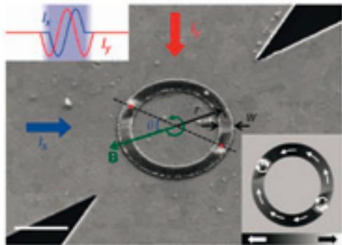
Fig.: Magnetization of a nanostructured permalloy ring.
