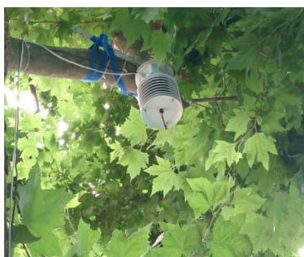
Fig. 4. Leaf surface temperature measurement: Photo of the measurement instrument, encased in a radiation shield, mounted on a branch, five meters above the ground (left). On the right the measured area, a dense leaf cluster, three meters below the instrument is shown.
