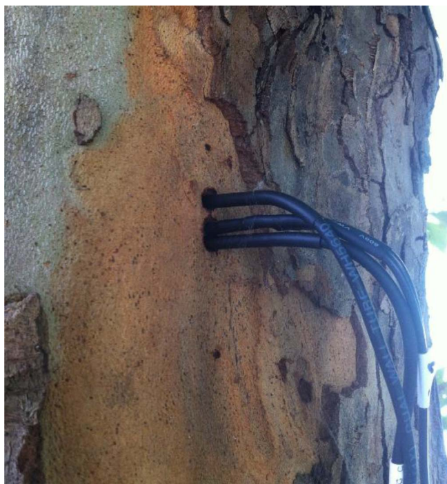
Fig. 3. Sap flow measurement: Photo of the two temperature probes placed above and below a heater probe into the sap wood (before insulation).
