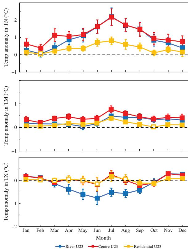
Figure 5. Temperature residuals between the historical thermometer locations and the current AWS station location. Monthly TX, TM and TN deviations including 95% error bars calculated over 2 years are shown. The residential values are an average of two sensors. Significant deviations are displayed as filled squares.
