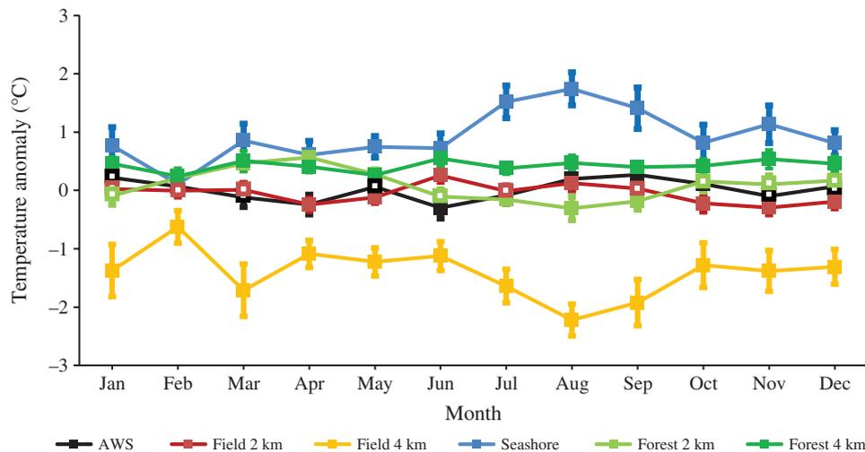
Figure 4. Seasonal pattern of temperature deviations recorded at Haparanda sensors over 2 years. Monthly temperatures are shown as anomalies from the mean of all sensors. Error bars display the variance as 95% confidence intervals. Filled squares mark significant deviations.
