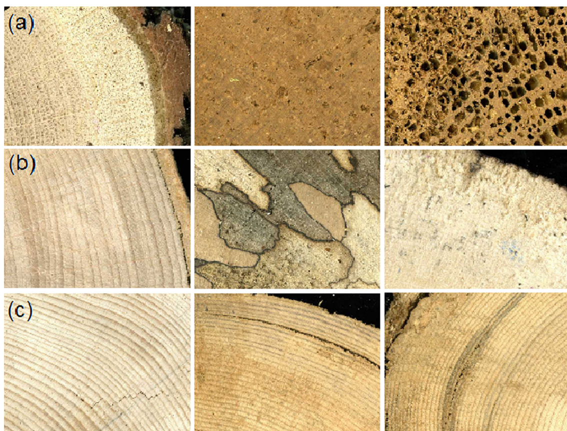
Fig. 2 Samples of CWD of Sessile oak (a), European beech (b) and Norway spruce (c) with increasing stages of decay
