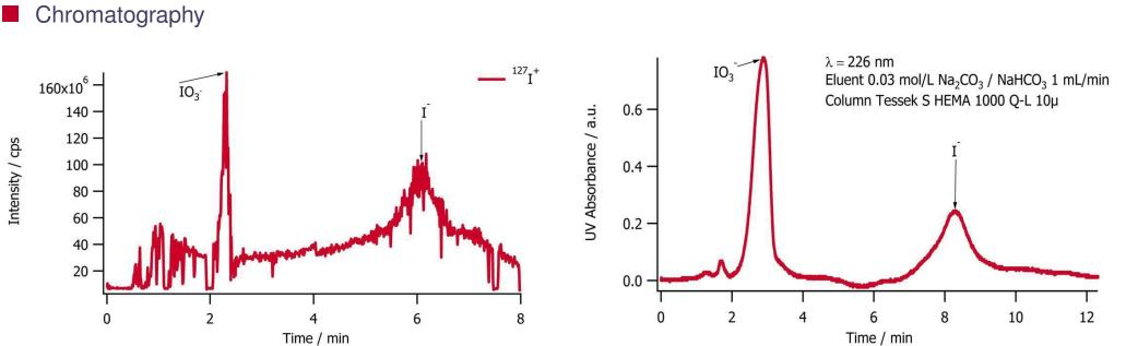
Figure 2: Separation of iodine and iodate - DOD-ICP-MS detection
