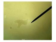
Figure 5: Microscopic images of dried residues dispensed by a microliter pipette (500 nl droplets, transferred mass: 500 pg Se).
