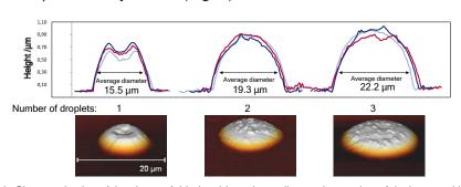
Figure 3: Characterization of the shape of dried residues depending on the number of dosing repetitions: (top) cross-sections, (below) AFM images.
