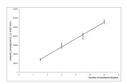
Figure 4: (left) TXRF-signal intensity per dosing event (9 replica) versus the delay between two events; (right) TXRF calibration curve: intensity versus number of transferred droplets (delay time 45 s).
