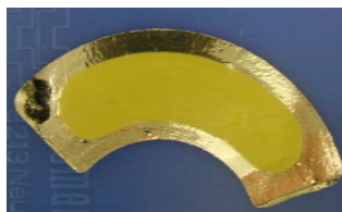
Figure 1: ^{238}\text{U} -target (265 \mu\text{g}/\text{cm}^2 ) produced by molecular plating of uranyl-nitrate from isobutanol solution.
