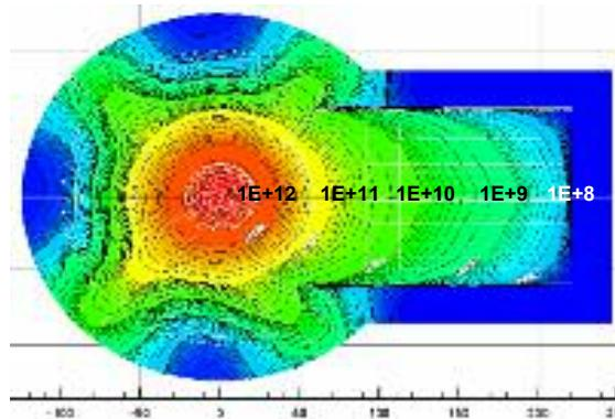
Fig. 3: Comparison between simulation and measurements using gold foils and TLDs in the thermal column
