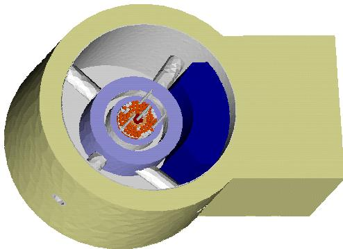
The calculations are validated measuring the neutron and gamma flux in the middle channel of the thermal column using gold activation foils and Thermolumineszenz dosimeter (TLD). Cadmium covered gold foils were used to separate the thermal and epithermal neutron flux. The irradiated foils were analysed using a standard high-purity germanium (HPGe)
