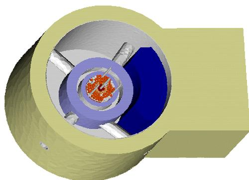
The calculations are validated measuring the neutron and gamma flux in the middle channel of the thermal column using gold activation foils and Thermolumineszenz dosimeter (TLD). Cadmium covered gold foils were used to separate the thermal and epithermal neutron flux. The irradiated foils were analysed using a standard high-purity germanium (HPGe)
