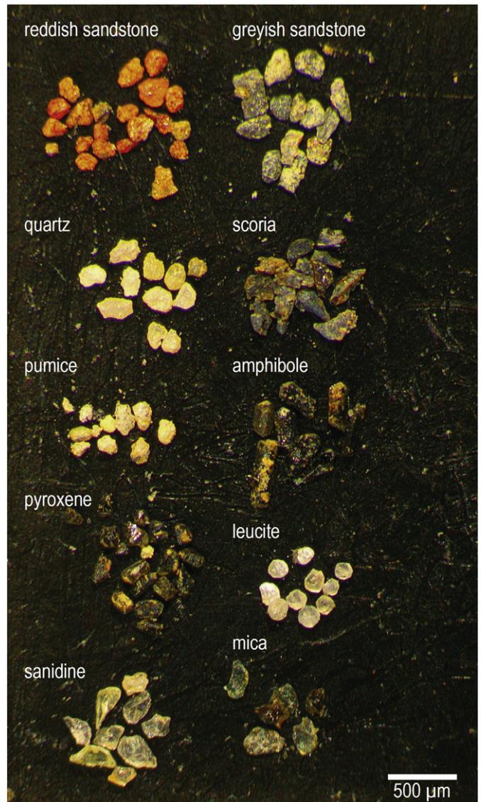
Fig. 2. Grains of the 250–125  $\mu$ m fraction in tephra layers as seen in the picking tray.
