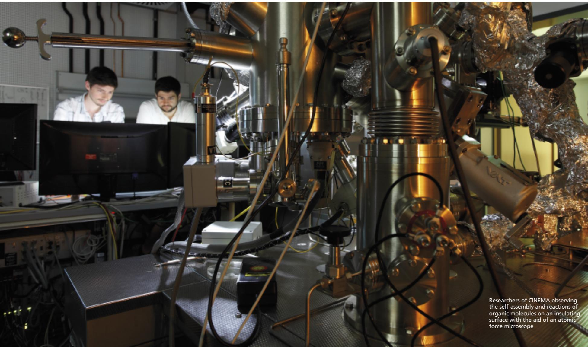
Researchers of CINEMA observing the self-assembly and reactions of organic molecules on an insulating surface with the aid of an atomic force microscope
