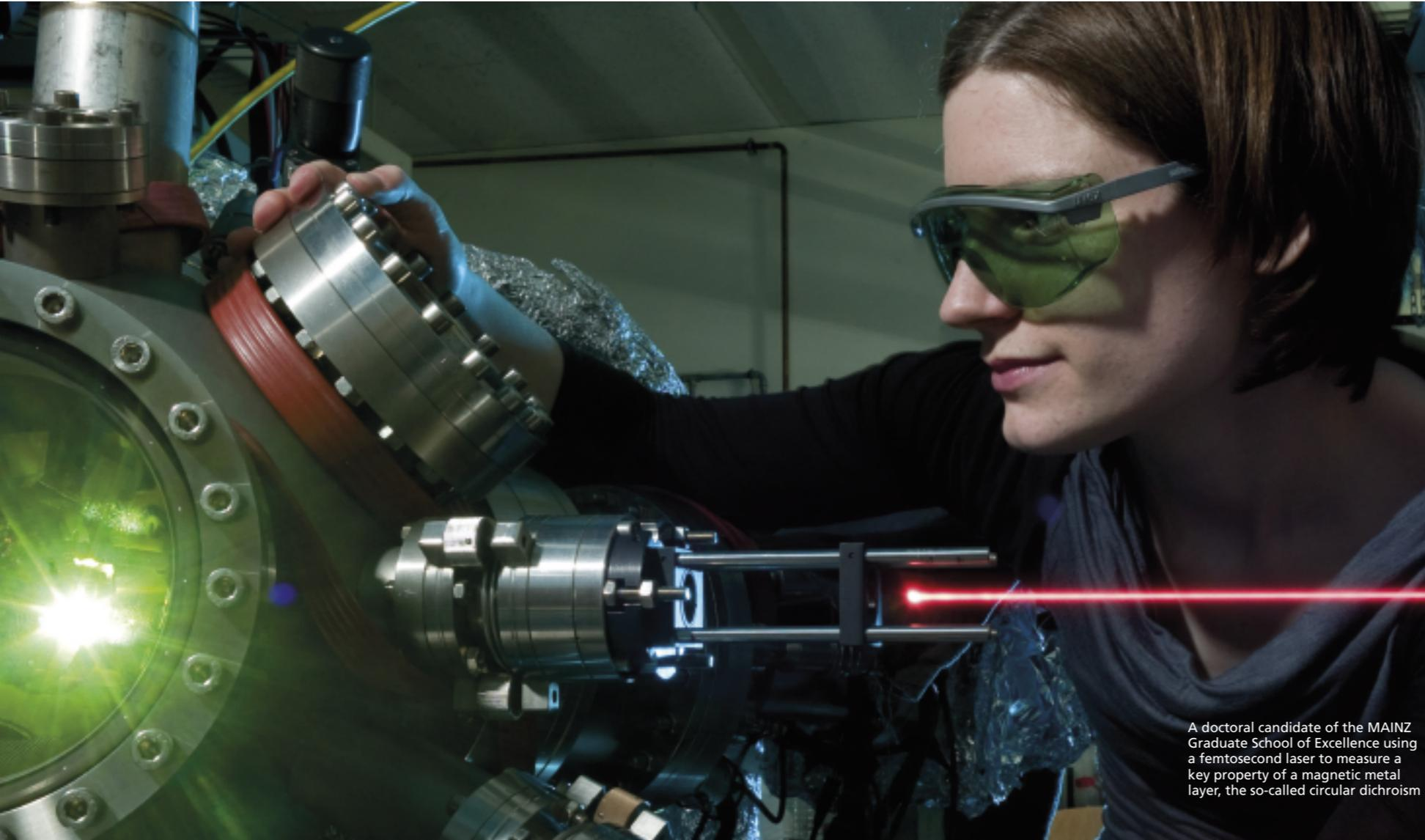
A doctoral candidate of the MAINZ Graduate School of Excellence using a femtosecond laser to measure a key property of a magnetic metal layer, the so-called circular dichroism
