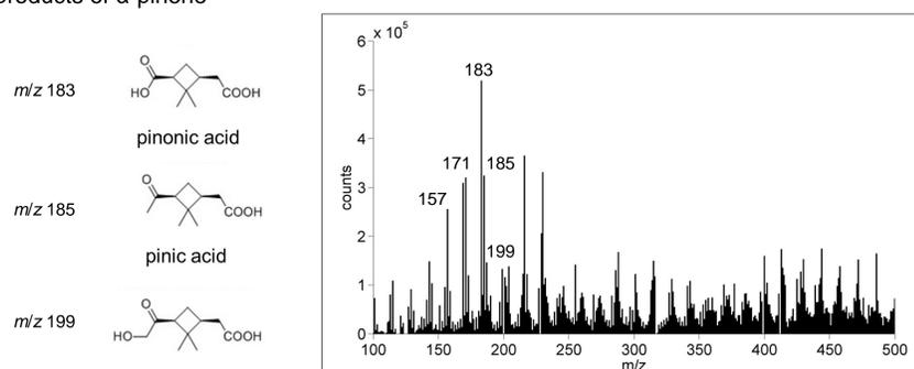
Figure 6: Mass spectrum in the negative ion mode of laboratory-generated SOA (background subtracted).
