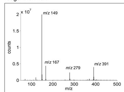
Figure 4: Background mass spectrum in positive ion mode: the four major signals correspond to plasticizers from the laboratory air which are known as common MS contaminants ( $m/z$  149 = phthalic anhydride ( $MH^+$ ),  $m/z$  167 = dimethyl phthalate ( $MH^+$ ),  $m/z$  279 = dibutyl phthalate ( $MH^+$ ),  $m/z$  391 = dioctyl phthalate ( $MH^+$ )).
