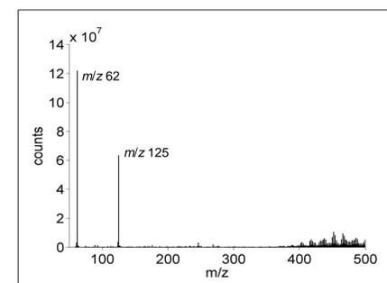
Figure 5: Background mass spectrum in the negative ion mode: the signals at  $m/z$  62 and  $m/z$  125 correspond to the formation of  $NO_2^-$  ions in the afterglow from ambient air. The signals at  $m/z$  ratios above 400 are probably caused by polymeric compounds from built-in plastics in the ion source assembly.
