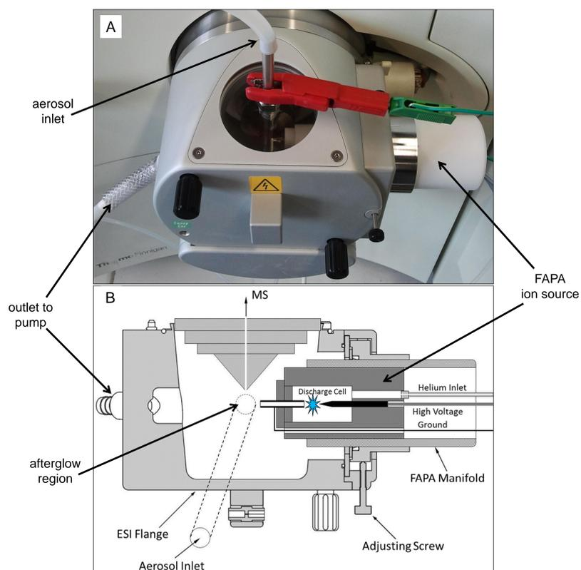
Figure 2: A) Photograph of the FAPA ion source mounted on a LQC Deca XP Plus (Thermo®) ion trap MS; B) Cross-sectional view of the FAPA assembly. The aerosol inlet is arranged orthogonal to the MS inlet and the FAPA exit. While the original Thermo® ESI flange was used the ESI manifold was replaced by a home-built FAPA manifold.
