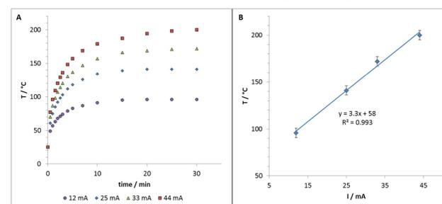
Figure 3: A) Maximum temperature of the afterglow region versus time for different current modes; B) Maximum equilibrium temperature at a chosen current.
