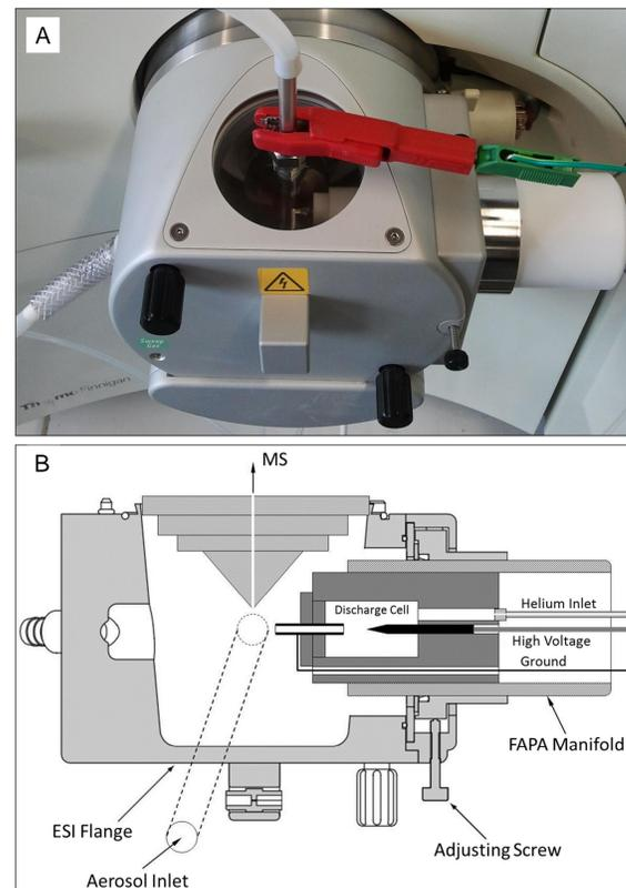
Figure 2: A) photograph of the FAPA ion source mounted on a LCQ Deca XP Plus (Thermo®) ion trap MS; B) Cross sectional view of the FAPA assembly. The aerosol inlet is arranged orthogonal to the MS inlet and the FAPA exit. While the original Thermo® ESI flange was used the ESI manifold was replaced by a home-built FAPA manifold.
