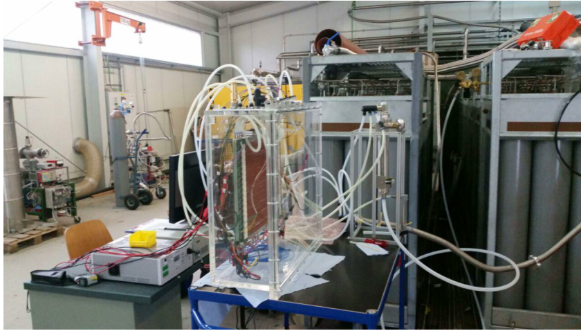
Figure 5.20.: Cooling setup with tracker module prototype and plexiglass enclosure. Image is taken from [130].
