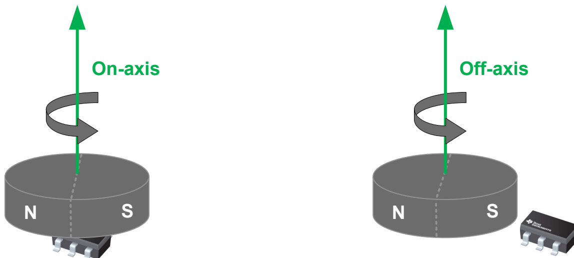
Figure 8-9. On-Axis vs. Off-Axis Angle Measurements
