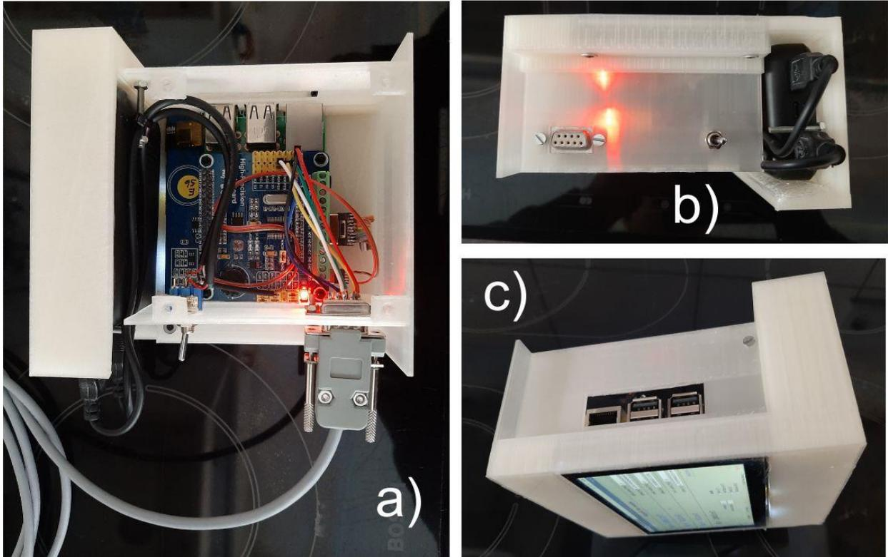
Fig. 15: The final device: a) view from the back (lying on screen). To the left (black box) is the powerbank connected via a regular switch to the USB power port of the Raspberry. To the right you can see my home-made HDMI/HDMI cable. B) Side view showing the D-Sub connector for the Hall-probes. C) shows the other side with the USB ports of the Raspberry.
