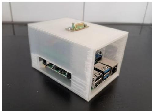
Fig. 16: Simple case for Raspberry and Waveshare-card. One can still attach the probes via a D-Sub connector on the top. Otherwise keyboard, mouse, screen and power supply still need to be attached.
