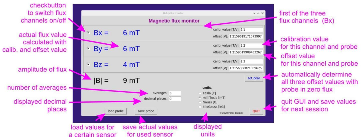
Fig. 12: The Hall-pi GUI with explanations.
