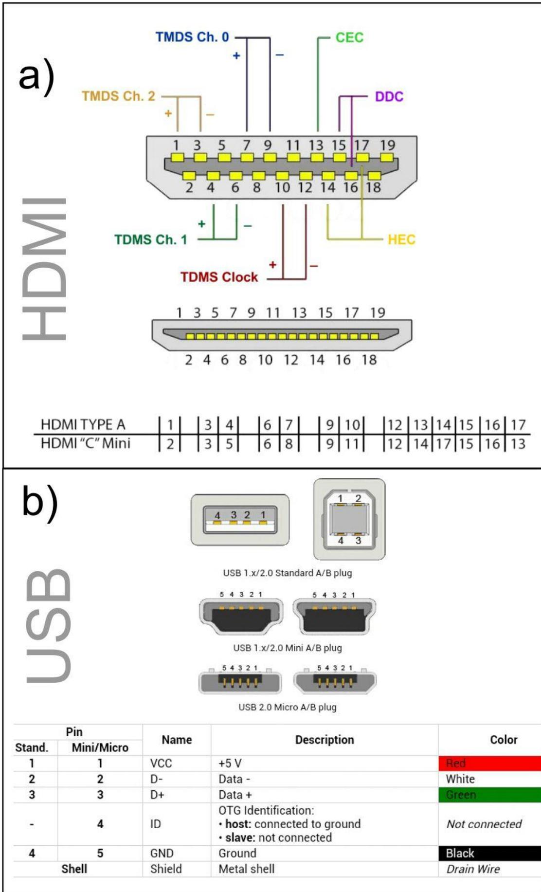
Fig. 14: Connections of a) HDMI and b) USB connectors.
