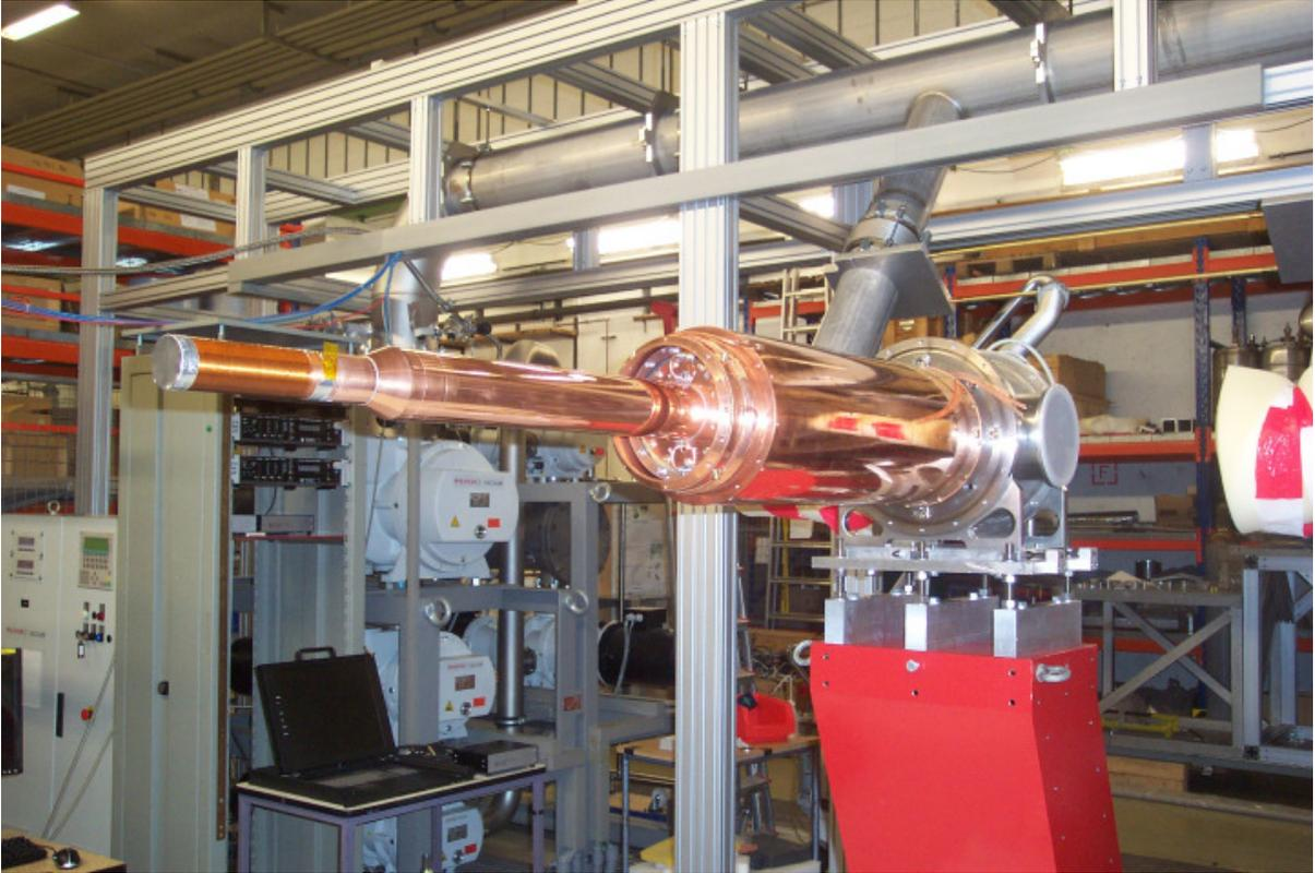
Figure 11: The dilution refrigerator for the Crystal Ball Frozen Spin Target.
