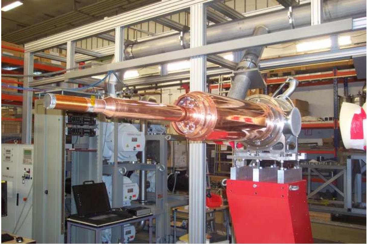
Figure 15: The dilution refrigerator for the Crystal Ball Frozen Spin Target.
