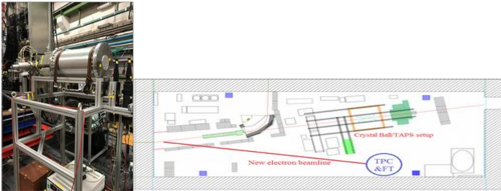
Fig.5. Plan of A2 hall. The ACTAR2 setup is installed downstream of the Cristal Ball/Taps setup. A temporary electron beam line was constructed for this test run. Also shown is a new electron beam line designed especially for this experiment.
