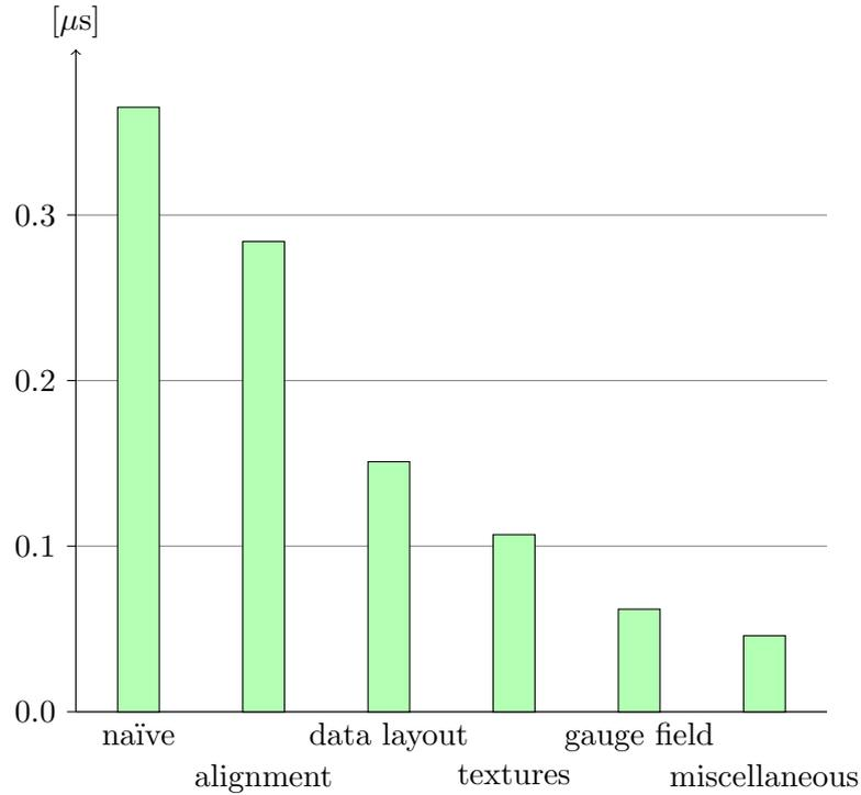
**Figure 5.6:** A symbolic synopsis of the progress and the impact of different optimization methods on the performance of the Wilson-Dirac operator. The lattice size was set to  $16^4$ . For a detailed explanation see the text.
