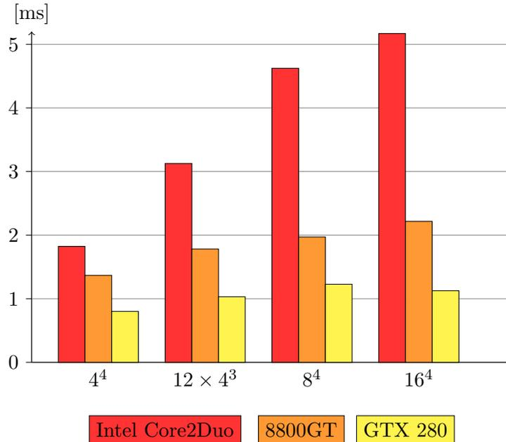
**Figure 5.5:** Calculation of the low-lying eigenvalues of the Wilson-Dirac operator. On the  $y$ -axis it is shown the runtime to calculate the low-lying eigenvalues and eigenmodes of the Wilson-Dirac operator. The time is normalized to the lattice volume and the number of eigenvalues found.
