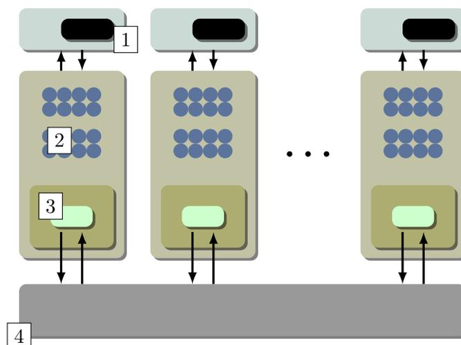
**Figure 3.1:** Simplified illustration of the shader core architecture of the NVIDIA G80 chip set. Up to 8 pairs of streaming multiprocessors are arranged on the chip, each consisting of (1) a instruction scheduler and the register file, (2) 16 scalar processors and (3) the texture fetching unit and the texture cache. Each multiprocessor has access to the (4) global memory.
