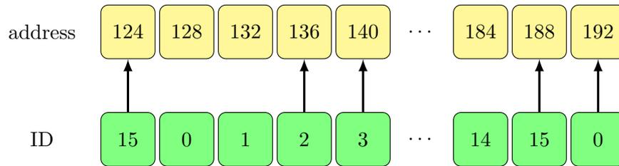
**Figure 3.4:** Example of coalesced access to global memory. Although not all threads in the half-warp participate in the memory access, a single memory instruction is issued because the memory access can be predicated.
