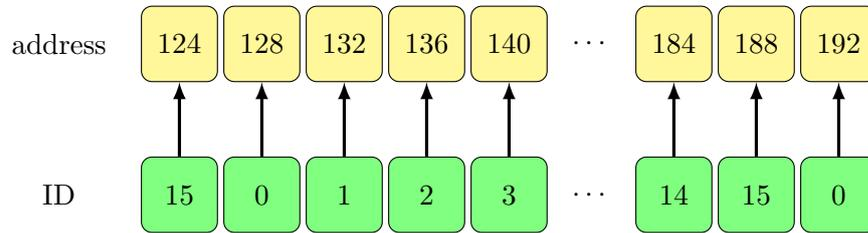
**Figure 3.3:** Example of coalesced access to global memory. All threads in a half-warp read one memory word in sequential order and the memory access is aligned to 32 byte and only a single memory instruction is issued. Coalescing would also be possible for 64 and 128 byte accesses.
