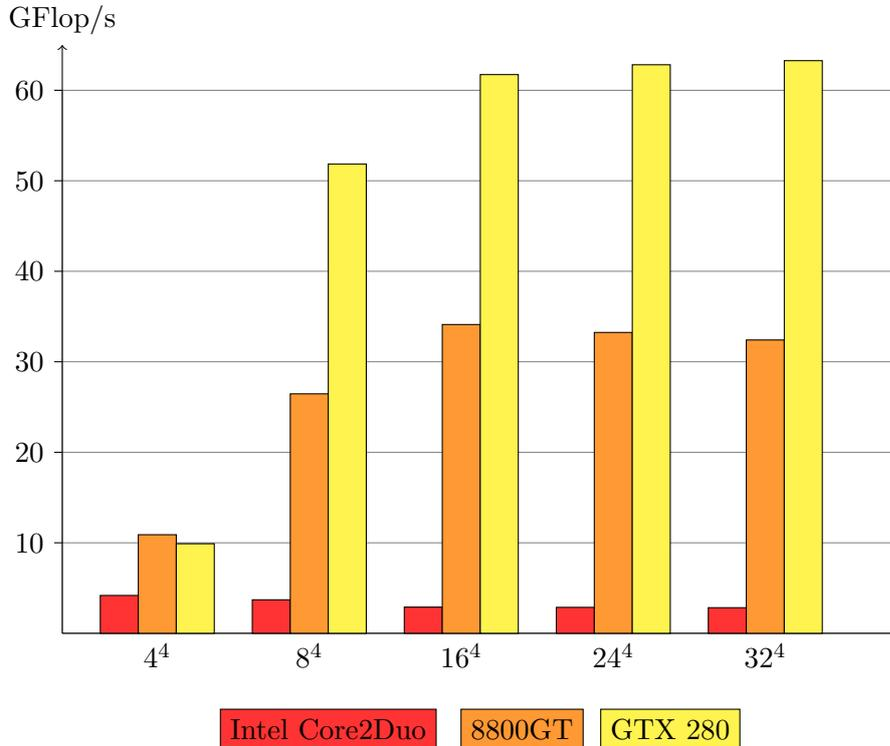
**Figure 5.2:** Effective floating-point operations per second for the Wilson-Dirac operator. The reconstruction of the gauge fields is not taken into account as the work necessary is not mandatory.
