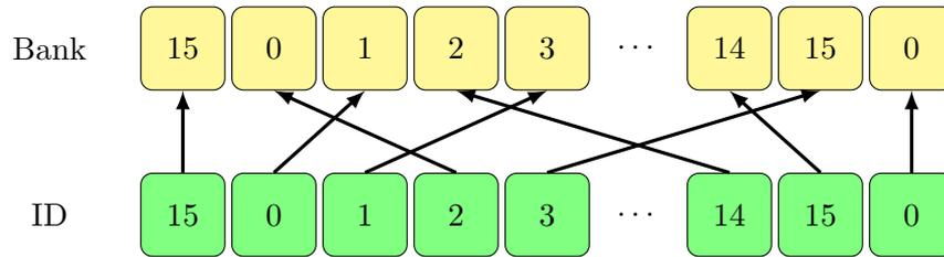
**Figure 3.7:** Example of access to shared memory without bank conflicts. Although the access is randomly distributed, all threads in the half-warp access a different memory bank.
