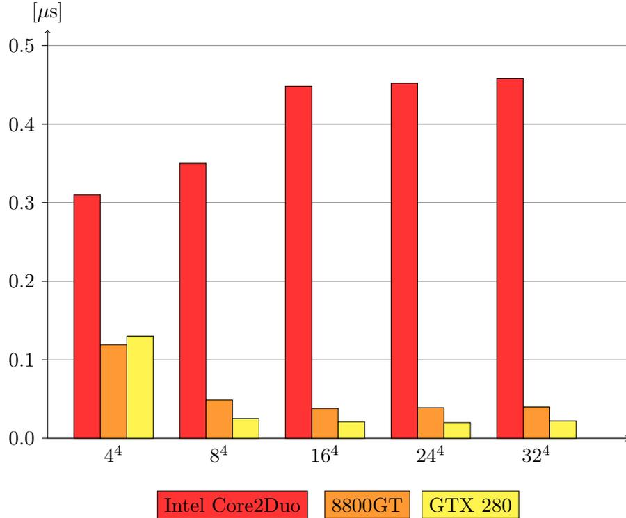
**Figure 5.1:** The execution runtime per lattice site of the Wilson-Dirac operator for different lattice volumes. Compared to the CPU implementation, the GPU implementation around 12 times faster for the NVIDIA 8800GT and around 22 times faster for the NVIDIA GTX 280. One noteworthy details is, that there is almost no volume dependence for the GPU implementation.
