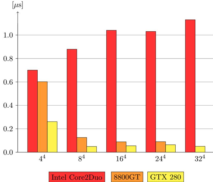
**Figure 5.4:** Execution runtime of the Neuberger operator without low-modes. On the  $y$ -axis the runtime of the evaluation for the Chebychev polynomial approximation of  $\text{sign}(Q)\eta$  in the Neuberger operator is shown. The runtime is normalized to the lattice volume and the degree of the approximating polynomial.
