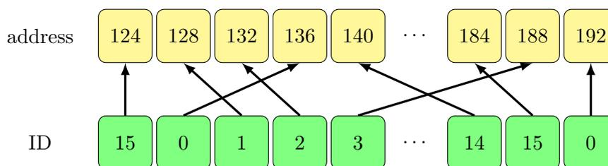
**Figure 3.5:** Example of uncoalesced memory access to global memory. Threads in the half-warp access global memory in random order which results in the maximum of 16 memory instructions.
