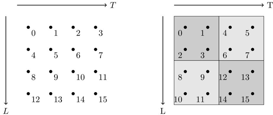
**Figure 4.1:** Left: The lattice sites are indexed in sequential order. It is easy to see that there are huge jumps for the memory addresses of adjacent lattice sites in the spatial direction. Right: Lattice sites get grouped into blocks. Inside the blocks, sites are indexed in sequential order. Huge jumps only occur between sites of different blocks.
