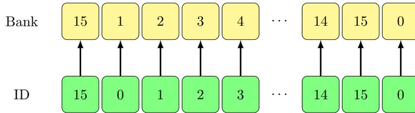
**Figure 3.6:** Example of access to shared memory without bank conflicts. Each thread in the half-warp accesses a different memory bank.
