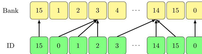
**Figure 3.8:** Example of access to shared memory with bank conflicts. Memory banks 3 and 14 get accessed multiple times by threads in the half-warp and therefore need to be serialized. However, both memory requests can be combined in a single broadcast, resulting in a two-way bank conflict.
