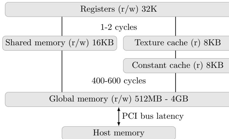
**Figure 3.2:** Hierarchical overview over the memory spaces available on the GPU. Memory spaces are ordered by access latency from the kernel from low to high latency times. For detailed description see the text.
