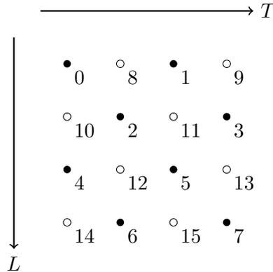
**Figure 4.2:** An even/odd-indexed lattice. Black dots are even lattice sites, white dots are odd lattice sites. From that scheme it is clear that even lattice sites are surrounded by odd sites only, and vice versa. That way, jumps for the memory addresses can be avoided almost completely.
