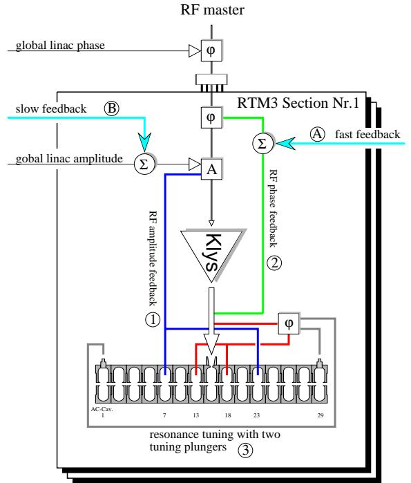
Figure 2: RF-feedback of RTM3. For clarity neither all 5 accelerating sections nor all 29 AC-cavities of a section are shown.
