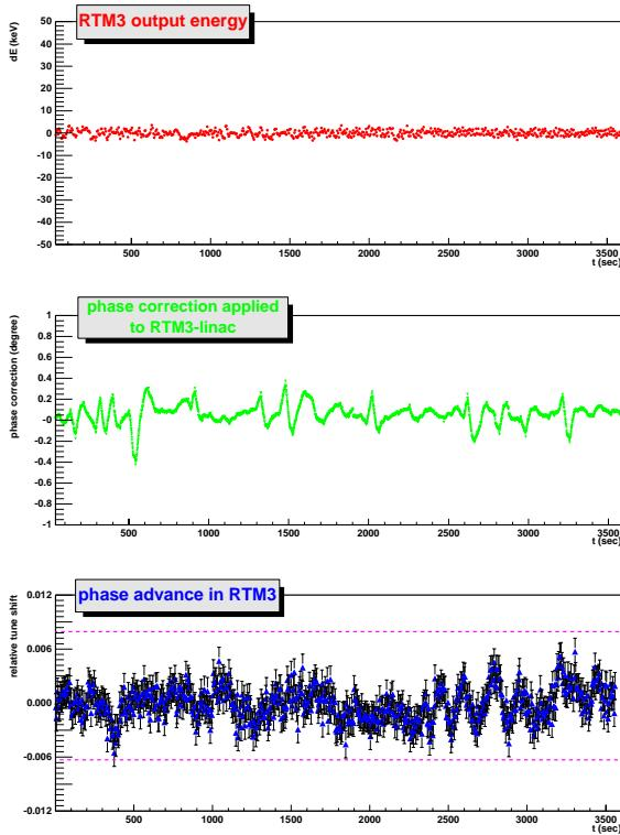
Figure 5: Both loops in action at  $2.5\mu\text{A}$  under favourable conditions, i.e. the longitudinal tune does not demand any correction of the linac amplitude.
