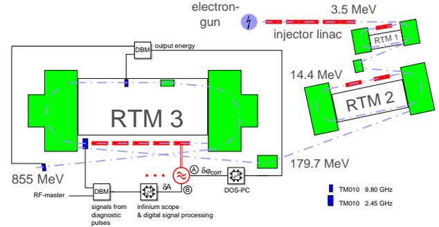
Figure 1: The Mainz Microtron cascade. (A): fast feedback loop. (B): slow feedback loop.
