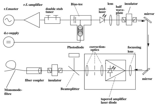
Figure 1: Set-up of Laser-system
