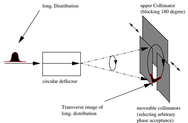
Figure 3: Principle of bunch length measurement
