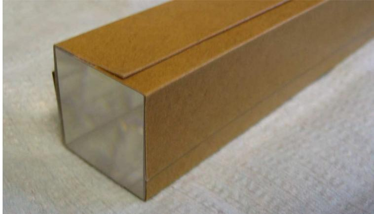
**Figure 4.5:** Detail of one crystal wrapped in reflective foil.
