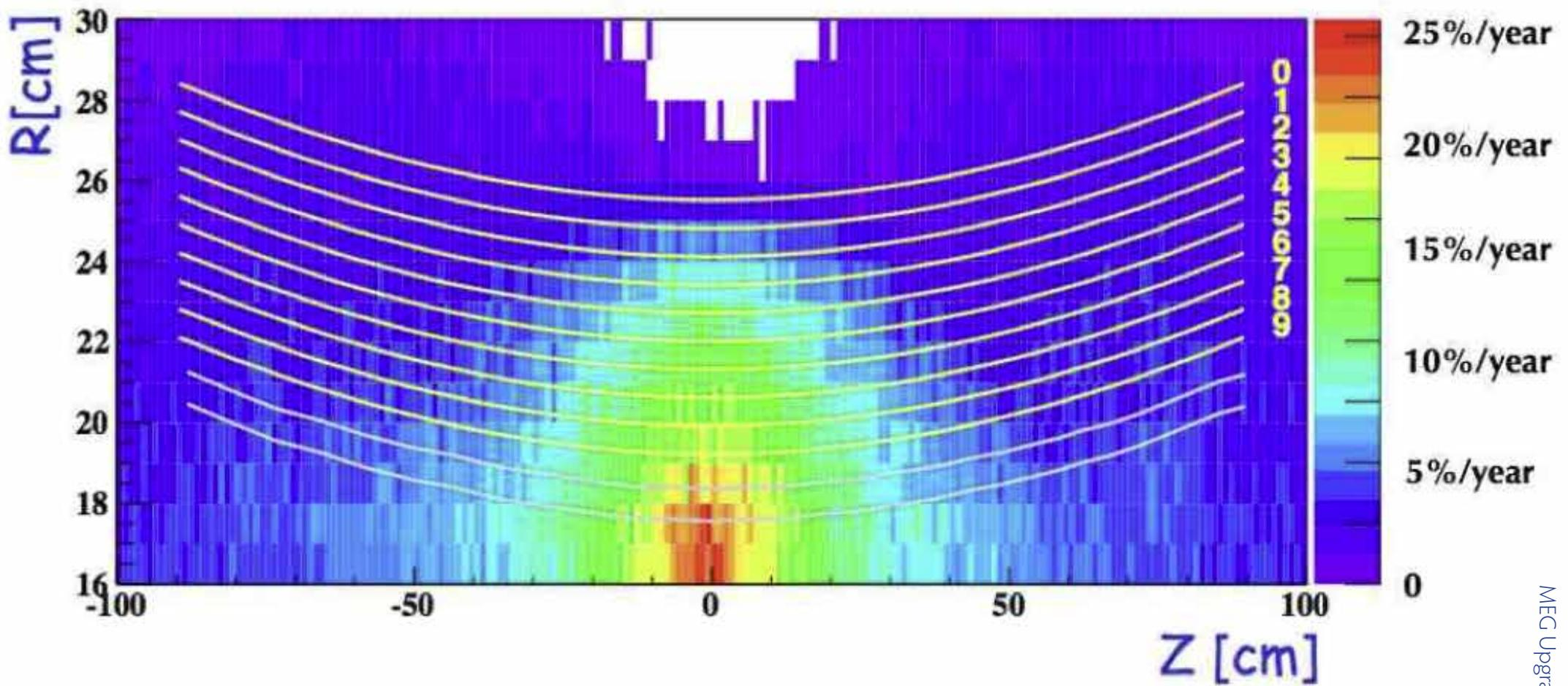
FIG. 24: Gain drop in 1-year of DAQ time at  $7 \times 10^7 \mu^+/\text{sec}$ .
