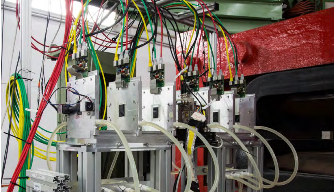
Figure 4.1: Picture of a EUDET telescope with a MUPiX prototype as device under test.
