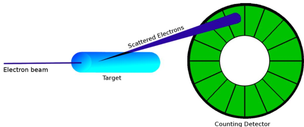
Beam :  $E_{beam} = 150 \text{ MeV}$ ,  $I_{beam} = 150 \mu\text{A} = 10^{15} e^- / \text{s}$ ,
