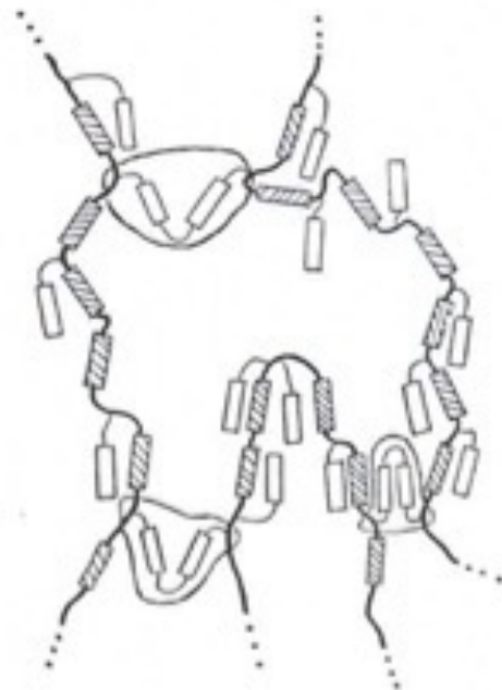
Fig. 9.27: Schematic drawing of networks prepared from side group, main chain and combined main chain/side group polymers [27].
