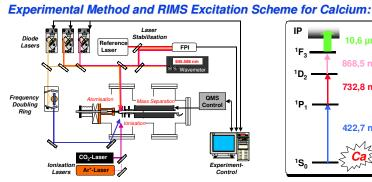
The setup for high resolution RIMS [2] consists of three major components:
